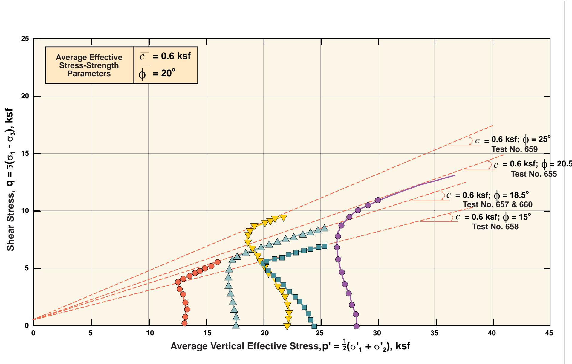
Plate GDR 79-2b: Effective Stress Paths from Triaxial Compression Tests on Melange Matrix
