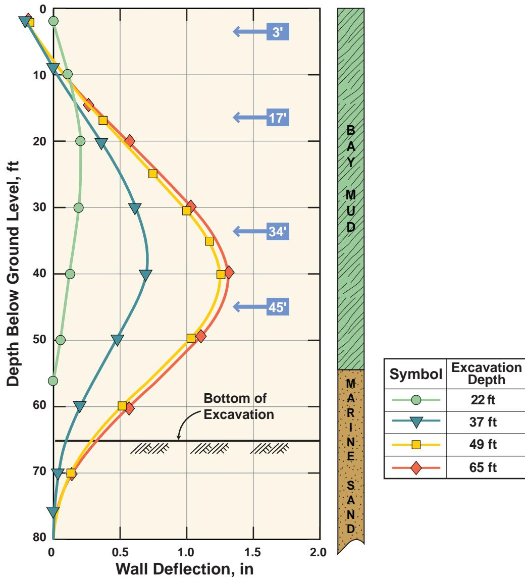
Plate H-01: Wall Deflection at Various Stages of Excavation
