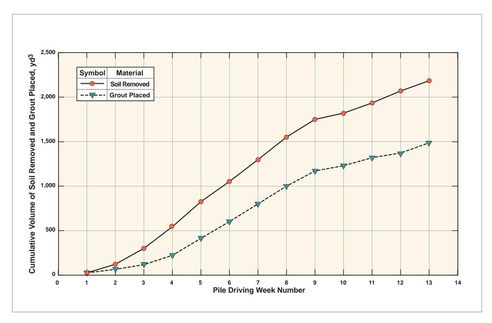
Plate B-02.2: Cumulative Removal of Soil/Placement of Grout VS. Pile Driving Week W:\Infrastructure\Geotech\UC Berkeley 2008 Seminar\Preliminary\Plate B-02.2
