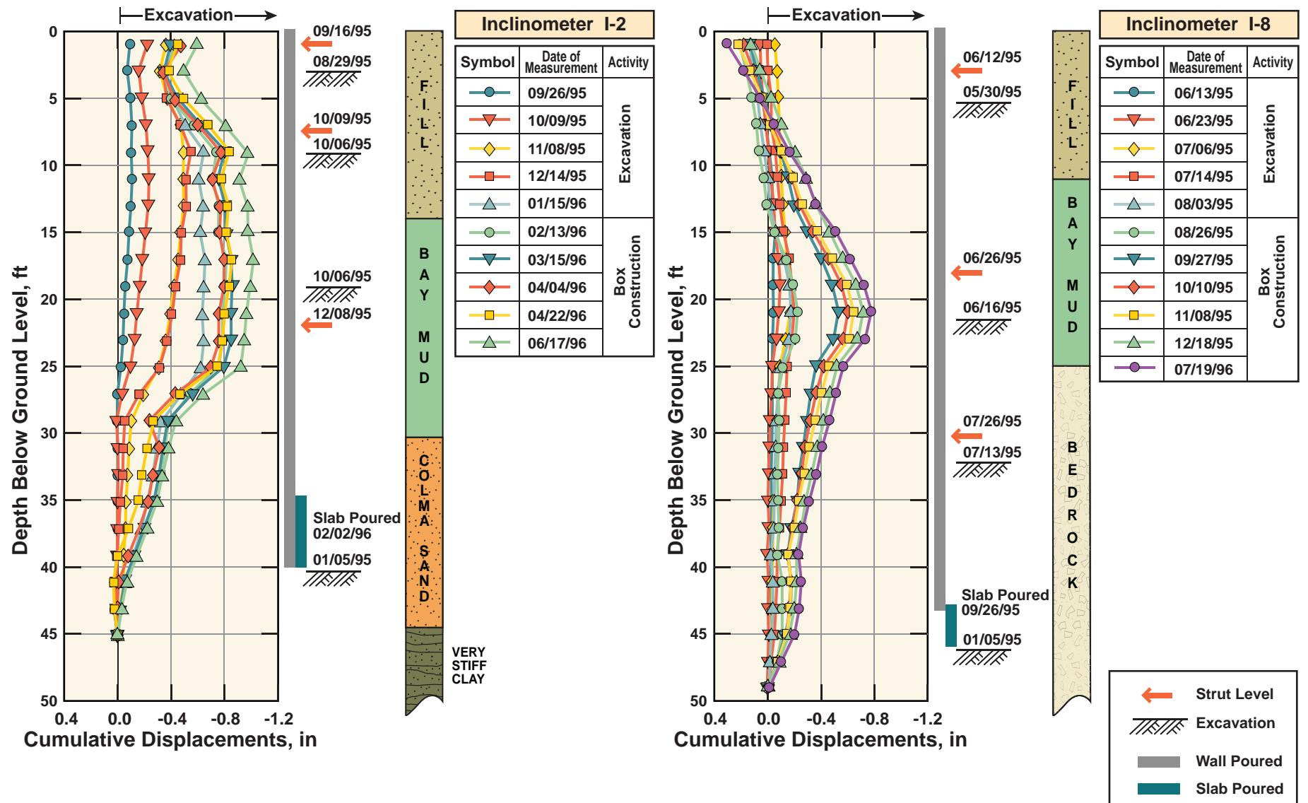
FIG\_253: Lateral Deformations Caused by Excavation and Box Construction: Islais Creek Contract B
