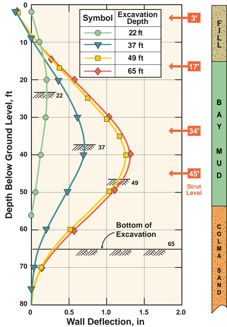
FIG\_249: Bay Mud Strengths and Excavation Deformations: Rankin Pump Station
