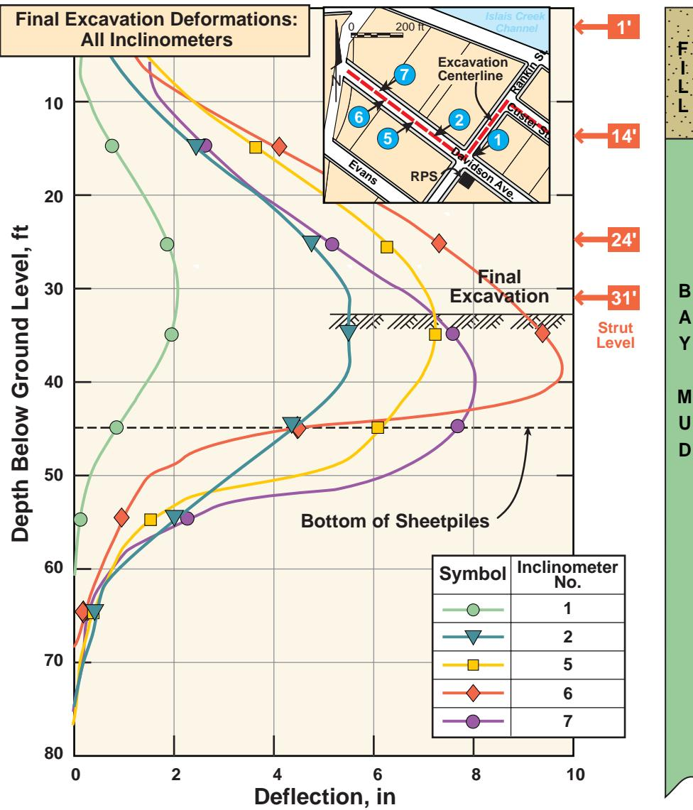
**FIG\_247C: Excavation Deformations: Davidson Street Sewer and Ranking Pump Station**
