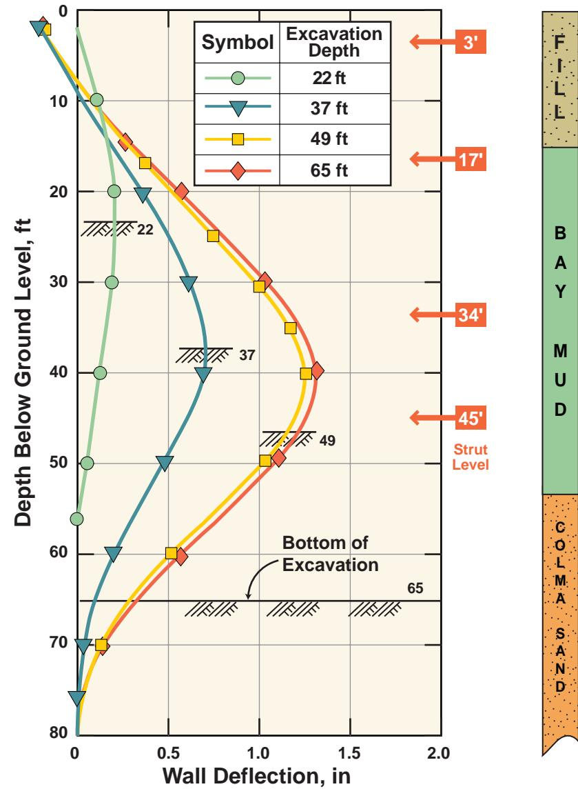
FIG\_247B: Excavation Deformations: Davidson Street Sewer and Ranking Pump Station
