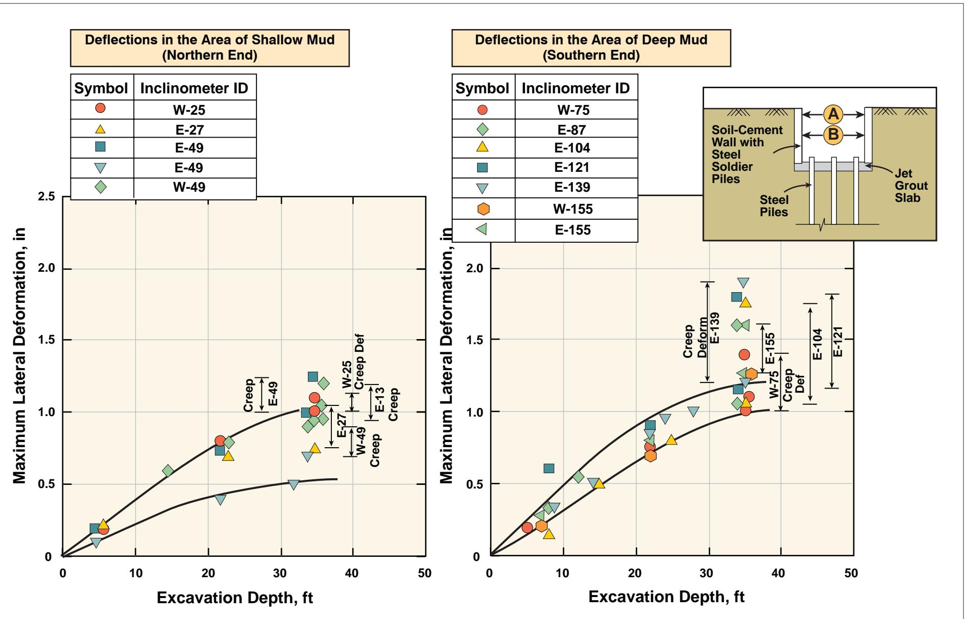
FIG\_241: Lateral Deflections Versus Excavation Depth: Excavations Along Indiana Street: Islais Creek Contract D
