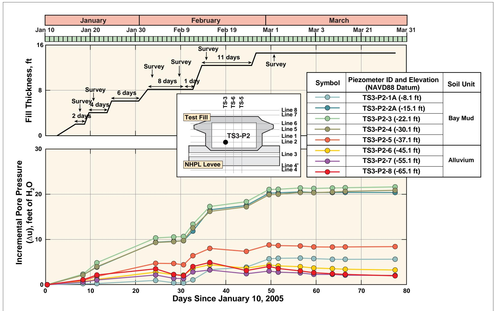
FIG\_155: Excess Pore Pressures Versus Time Measurements Under the Fill Instrument Line No. 2, Section No. 3
