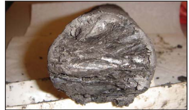
Picture 3: View of core cross-section illustrating irregular contacts between different materials, and laminated structure.
