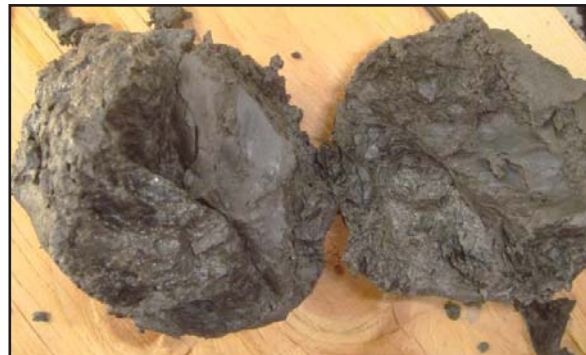
Picture 5: Close-up view illustrating evidence of shear deformations and slickensides.
